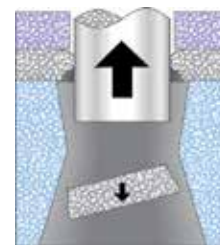
Punch retracts and slug is free to fall down and away through exit taper of the Slug Free® die.
